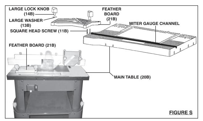
3. **NOTE:** The Feather Boards (14C, 21B) are designed to hold the workpiece in place and prevent kickback. To adjust the Feather Boards, simply loosen the Lock Knobs (8C, 14B) and move the Feather Boards into the workpiece. Then, retighten the Lock Knobs. Make sure the "feathers" of the Feather Boards allow easy feed of the workpiece and help prevent kickback. (See Figures R and S.)
